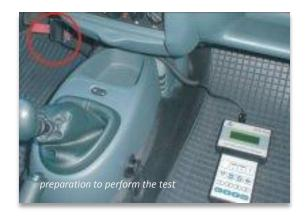
The AMX520 and AMX520/M (A-meter\*) allow to test break effectiveness of vehicles like trucks,
